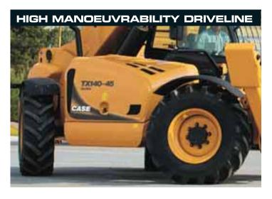
TX machines are incredibly agile, moving rapidly about the site thanks to a four-speed Powershift transmission and the easy to use three mode steering system. This combination of proven components ensures that there is no costly heat build-up in the transmission, even when travelling at high speeds on the road, where permitted.
