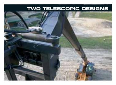
The TX range uses robust telescopic booms with inherent rigidity and strength to allow many hours of safe lifting. The TX130-33 has a chain driven extension for the second boom section, while all larger machines use an internally mounted hydraulic twin cylinder to extend the boom. All models are equipped with safety valves on the lift, tilt and stabiliser cylinders, to prevent the boom dropping in the case of hose failure.
