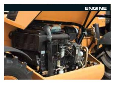
The TX telescopic handler range is powered by a 4.5 litre Case turbo engine. All machines are equipped with a low emission Tier III climate friendly engine, that with turbocharging and aftercooling offers from 99 hp to a healthy 118 hp and a powerful 516 Nm of torque.
