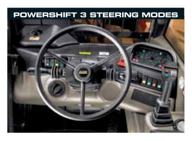
A proven Powershift transmission delivers four forward and three reverse speeds, with no heat build up despite high manoeuvring speeds. Working in combination with the flow sharing hydraulic system, the Powershift transmission offers precise control with high tractability, ideal for use on hard standing or in tough construction project conditions.
