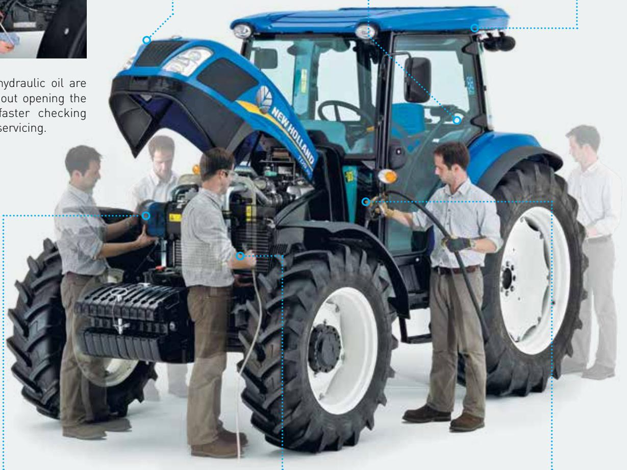
Check, clean or replace the air filter quickly and easily by undoing just four clips.
