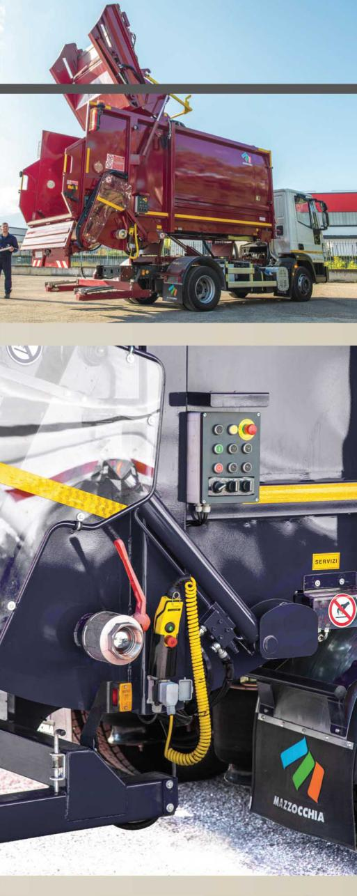
**THE MINICOMPACTORS MINIMAC\_B and POCKET\_B** are "UNIBODY" type, therefore the compaction system is contained within the body. The body forms a single collection tank.
