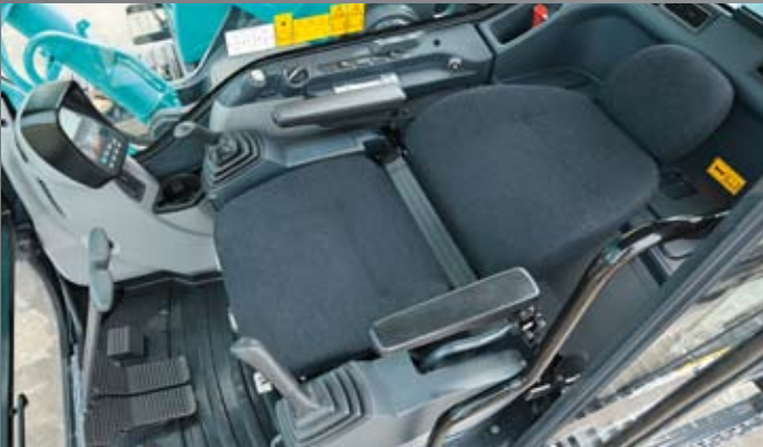
Seat can be reclined to horizontal position
