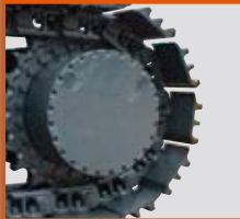
Stronger casing for travel motor
