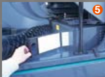
Air conditioner filter can be easily removed.
