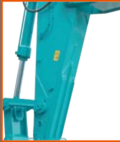
Reinforced arm with rock guard
