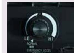
If unexpected trouble is experienced with the ITCS mechatronic control system, the machine can still be operated using the emergency acceleration system. Digging modes are also automatically relayed to an emergency system so that digging can continue with minimum down time.
