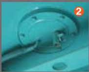
Fuel drain valve
