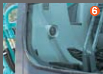
Hour meter can be checked while standing on the ground.
