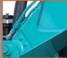
Reinforced boom side panels
